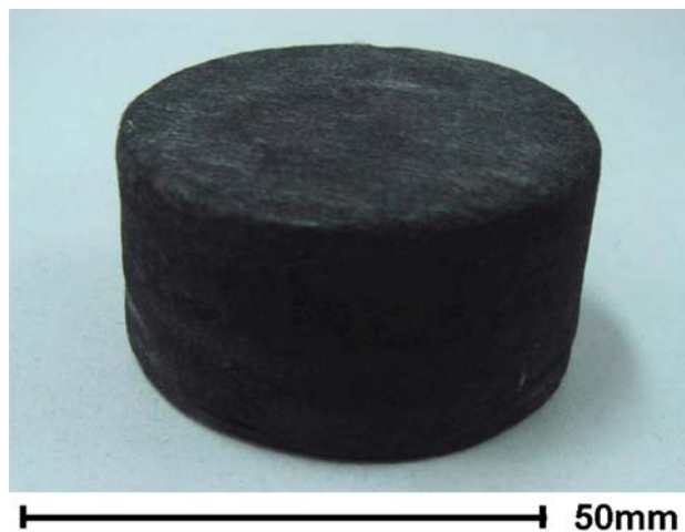
Fig. 3 The profile of the prepared short carbon fiber preform
